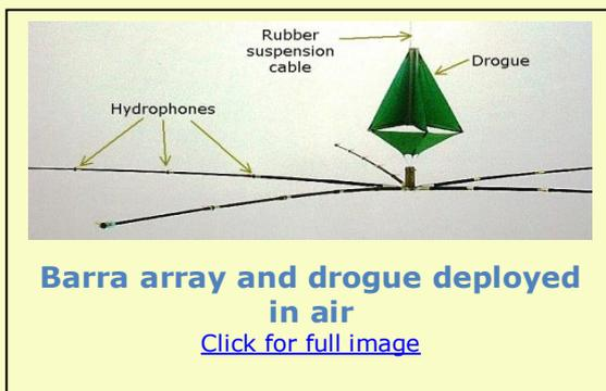
To isolate the hydrophone(s) from the movement of the surface buoy, sonobuoys commonly use compliant (rubber) suspension cables that contain the necessary electrical conductors. To increase further the degree of isolation, Barra uses a drogue to anchor the array to the water at depth. The large effective mass of the array, the drogue and the compliant cable together provide the desired isolation.
